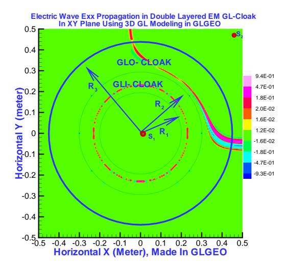
FIG. 3: (color online) At the time step 58*dt*, the *First electric wave*,  $E_{xx,1}$ , is propagating inside the inner layer,  $R_1 \leq r \leq R_2$ , and becomes very slow. The part of the front of *Second electric wave*,  $E_{xx,2}$ , has been inside of outer layer,  $R_2 \leq r \leq R_3$ , and being backward bending
