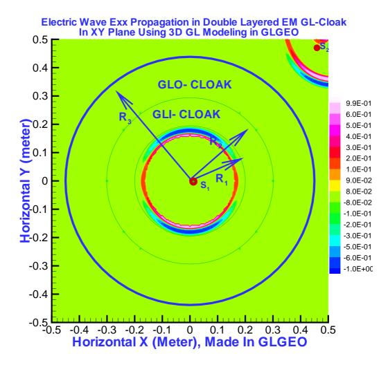
FIG. 1: (color online) At time step 18*dt*, the wave front of the *First electric wave*,  $E_{xx,1}$ , propagates inside the concealment  $r < R_1$ . The front of *Second EM wave*,  $E_{xx,2}$ , is located in free space, the right and top corner outside of the whole GL double layer cloak.
