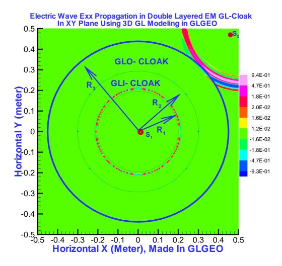
FIG. 2: (color online) At this moment of the time step 30dt, the front of the *First electric wave*,  $E_{xx,1}$ , propagates enter to the inner layer,  $R_1 \leq r \leq R_2$ ; the front of *Second electric wave*,  $E_{xx,2}$ , reaches the outer boundary  $r = R_3$  of the GL double layer cloak.
