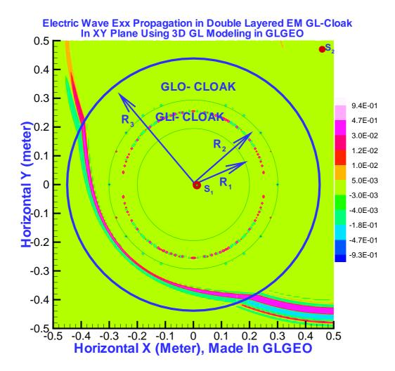
FIG. 5: (color online) At time step 98*dt*, one part of front the *Second electric wave*,  $E_{xx,2}$ , is propagating inside of the outer layer,  $R_2 \leq r \leq R_3$ , and around to other side far source. It is a little forward bending. The *First electric wave*,  $E_{xx,1}$ , is still propagating inside the inner layer,  $R_1 \leq r \leq R_2$ .
