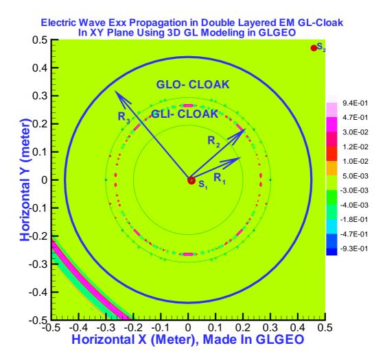
FIG. 6: (color online) At time step 128*dt*, the Second electric wave,  $E_{xx,2}$  has propagated outside the GL double layer cloak, a small part of its wave front is located in the left and low corner of the plot frame, which never be disturbed. The First electric wave,  $E_{xx,1}$ , is still propagating inside the inner layer,  $R_1 \leq r \leq R_2$ .
