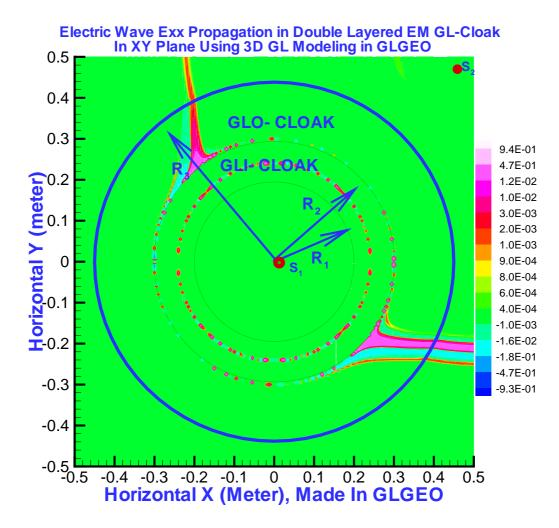
FIG. 4: (color online) At time step 75*dt*, the *Second electric wave*,  $E_{xx,2}$ , is propagating inside of the outer layer,  $R_2 \leq r \leq R_3$ , and around the shell  $r = R_2$  and never penetrate into inner layer and concealment,  $r < R_2$ . It does split into the two phases around the shell  $r = R_2$ . The *First electric wave*,  $E_{xx,1}$ , is propagating inside the inner layer,  $R_1 \leq r \leq R_2$ .
